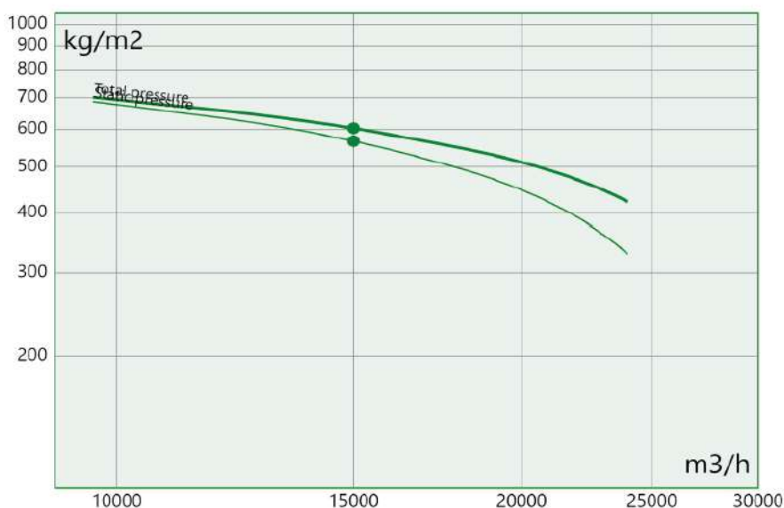
Chart relative to air at 0 °C - altitude 0 m - ρ = 1.292 kg/m 3
