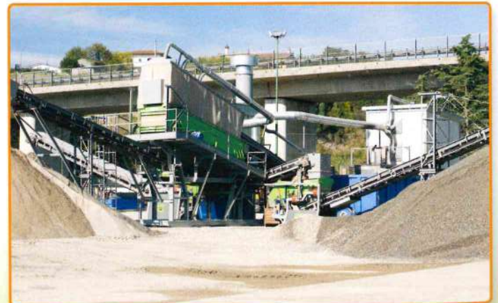
"Tornado" machinery coupling for treatment of different aggregate grain sizes (aggregates crushing plant for construction and demolition).
